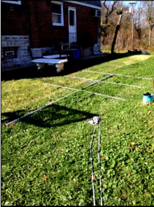
The 6m Telerex beam is in good shape for its next deployment.
